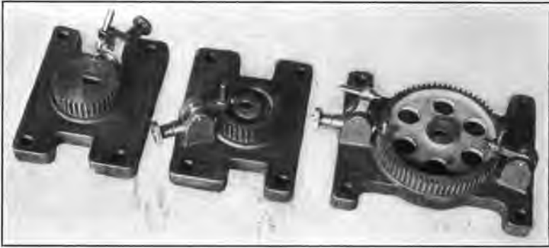
FIG. 152.—Gear keyseating and marking fixtures.
